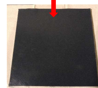
Used as a low cost filler in a compression molded polymer sheet
