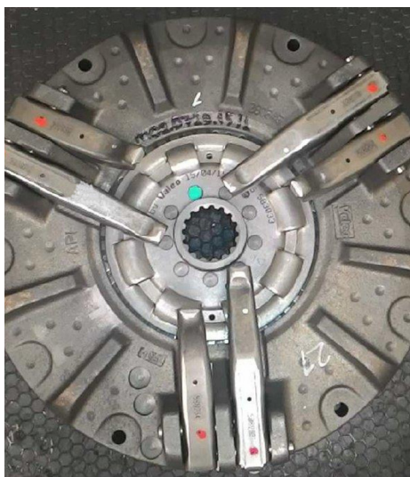
FRONT AND REAR OF NEWLY DESIGNED TRACTOR CLUTCH USED IN FIELD TESTS
