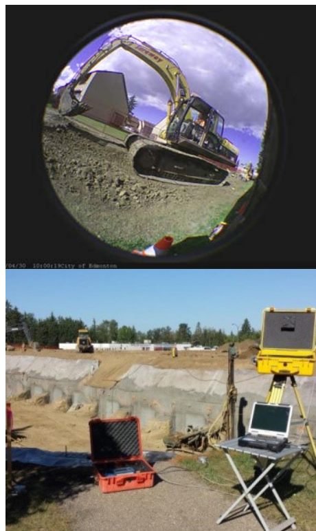
TOP PHOTO: INSTANTANEOUS PHOTO CAPTURE OF A TRIGGER VIBRATION EVENT. BOTTOM PHOTO: MONITORING VIBRATION LEVELS AT A CONSTRUCTION SITE WITH PHOTO CAPTURE.
