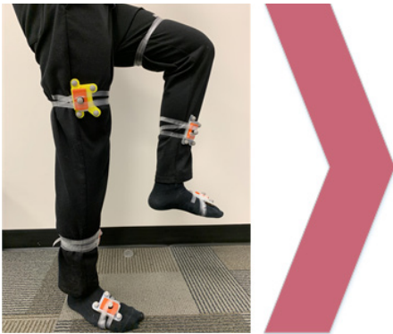
FIG. 1: BODY MOTION MEASUREMENT USING WEARABLE SENSORS.
