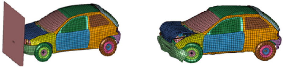
FIG. 2: AN AUTOMOBILE DESIGN PROBLEM WITH 124 VARIABLES AND 68 SIMULATION-BASED CONSTRAINTS CONSIDERING CRASHWORTHINESS, NOISES, VIBRATION, AND DURABILITY.
