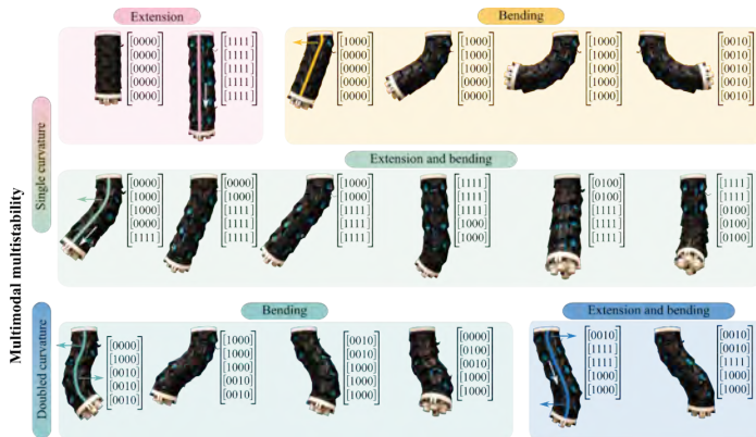
FIG. 1: MULTIMODAL MULTISTABILITY OF A SOFT ROBOTIC ARM AND ALTERNATIVE CATEGORIES OF ACHIEVABLE STABLE TRAJECTORIES.
