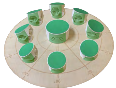
FIG. 3: BENT STABLE STATES ALONG EIGHT ORIENTATIONS ALIGNED WITH FOUR PLANES OF SYMMETRY OF THE CONSTITUTIVE MULTISTABLE UNIT CELL.
