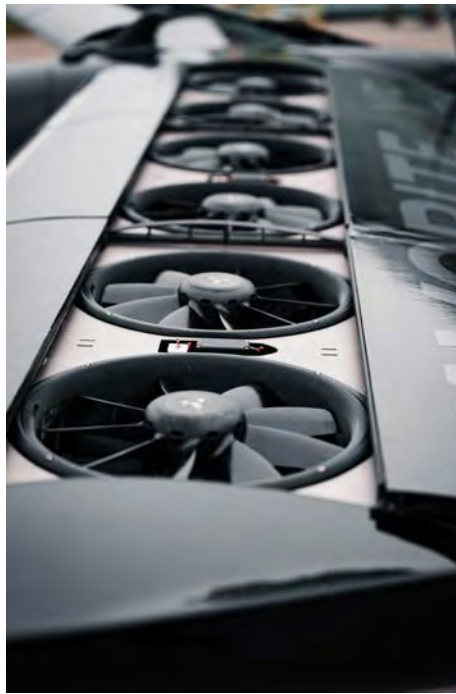
FIG. 2: PATENTED HOVR WING WITH ELECTRIC LIFT FANS.
