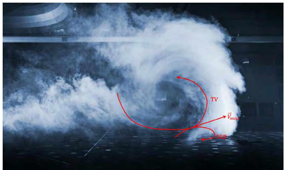
FIG. 1: FLOW VISUALISATION OF DOWNBURST VORTEX INTERACTION WITH THE SURFACE AT WINDEEE DOME. THE VISUALIZATION SHOWS THE RIGHT RADIAL SIDE OF THE DOWNBURST WITH TV THE TOROIDAL VORTEX, SRB THE SEPARATION-REATTACHMENT BUBBLE AND V_{max} THE MAXIMUM VELOCITY OCCURRENCE IN THE FLOW
