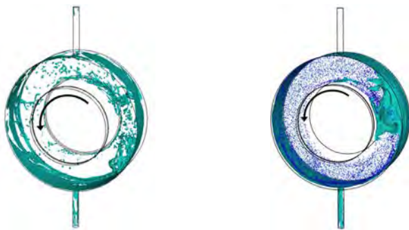
FIG. 1: ISO-SURFACE OF OIL VOLUME FRACTION \alpha_o = 0.3 USING TWO SEPARATE COUPLING TECHNIQUES TO TRACK DROPLETS.
