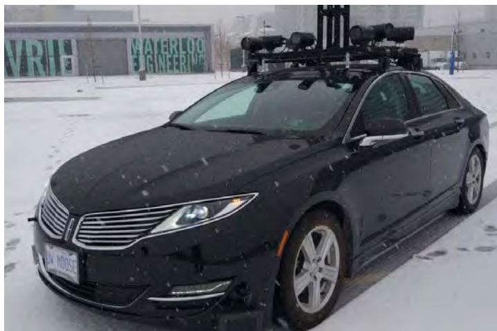
FIG. 1: THE AUTONOMOOSE AUTONOMOUS VEHICLE TESTING PLATFORM USED TO COLLECT THE DATASET ON SNOWY WINTER ROADS.
