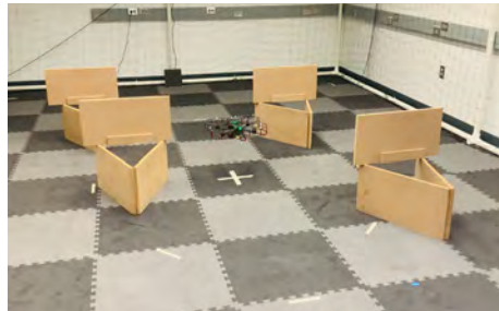
FIG. 1: EXPERIMENTAL TEST SPACE. LABORATORY 3-D FLIGHT TEST SPACE AND COLLISION-FREE WAYPOINTS. 3
