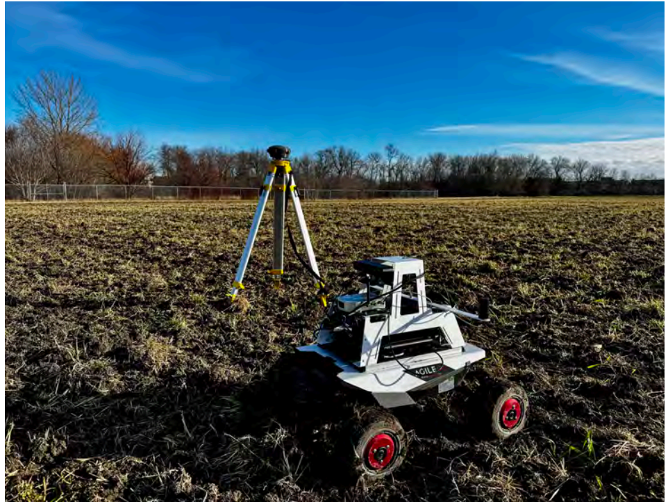
FIG. 2: AN AGILEX SCOUT MINI PLATFORM DURING OUTDOOR TESTING IN A PRAIRIE FIELD NEAR A SURVEY-GRADE RTK-GNSS BASE STATION. THIS SETUP IS USED TO EVALUATE NAVIGATION AND CONTROL PERFORMANCE UNDER UNEVEN TERRAIN AND REALISTIC LOCALIZATION CONDITIONS RELEVANT TO AGRICULTURAL FIELD ROBOTICS.
