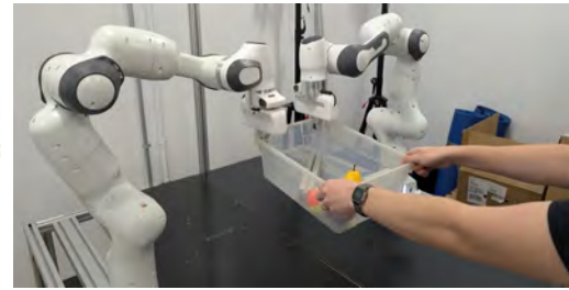
FIG. 2: FRANKA EMIKA ROBOT MANIPULATORS CO-MANIPULATING AN OBJECT WITH HUMAN.
