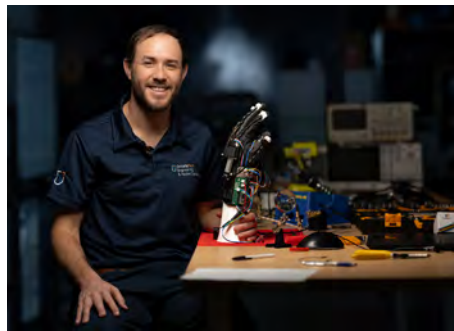
FIG. 1: DR. YURKEWICH DEMONSTRATING THE HERO GLOVE SOFT HAND EXOSKELETON AT THE ONTARIO TECH UNIVERSITY BIROBOTICS LAB.
