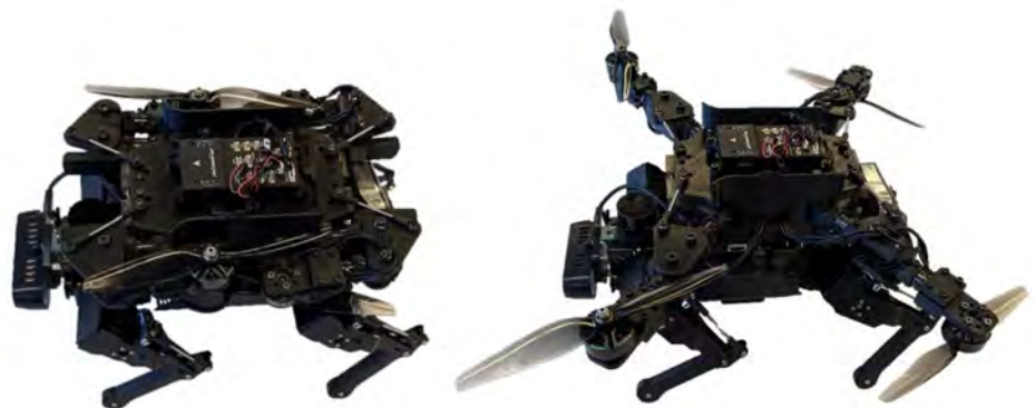
FIG. 3: PUGASUS PROTOTYPE: ARMS STOWED (LEFT) AND ARMS DEPLOYED (RIGHT).
