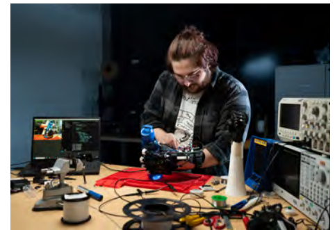
FIG. 2: DAIMEN LANDORI-HOFFMANN, MASC DEMONSTRATING THE HERO GLOVE GRIP FORCE AND COMPUTER VISION CONTROL SYSTEM FOR EVERYDAY TASK ASSISTANCE AND REHABILITATION.
