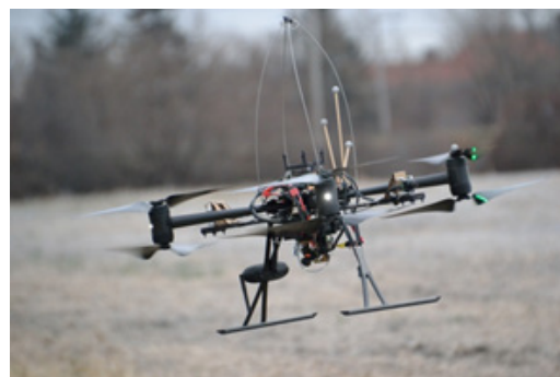
Draganflyer X8 unmanned aerial vehicle being tested outdoors.
